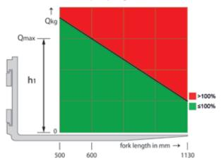
Qmax = 2500 kg @ 600 mm or limited by Qmax of the forklift truck
